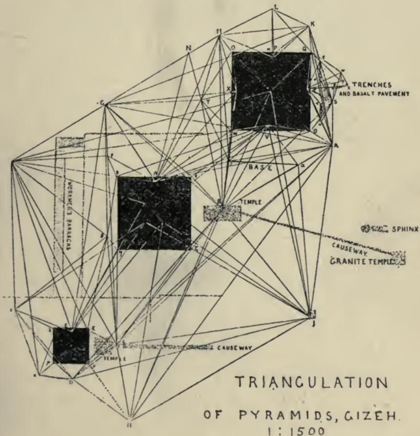
vations were repeated so many times, that if I finished the work at a single station in one day I was well satisfied. The result of all this mass of checked observations, after duly reducing and computing, was that there was scarcely a point about which one quarter inch of uncertainty remained, and most of the points were fixed to within one-tenth of an inch. These points
