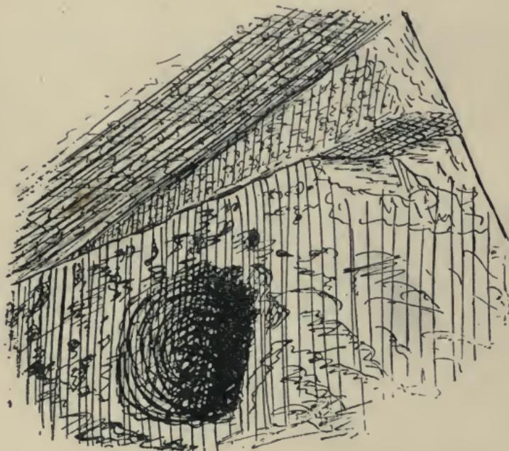
9. PIVOT HOLE OF DOOR AND CUTTING OF ROOF :
