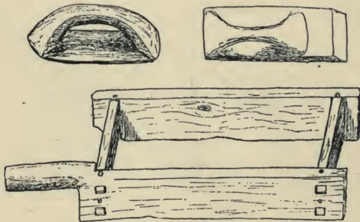
89. PLASTERERS' FLOATS, AND BRICK-MOULD.
