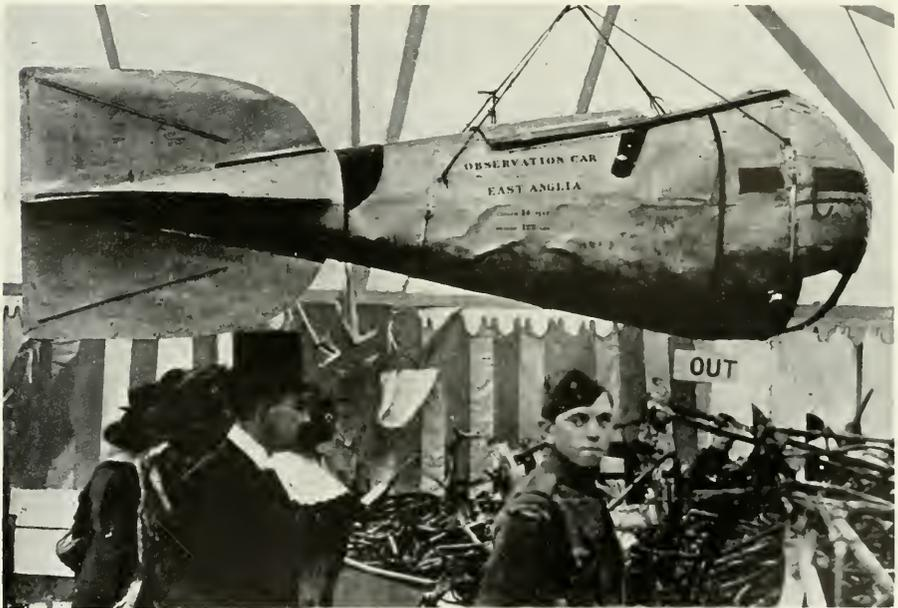
Zeppelin observation car. From a Zeppelin brought down in East Anglia: it is fourteen feet long, built of aluminium and weighs one hundred and twenty-two pounds. It was suspended by a wire cable 5,000 feet in length, through which ran a telephone wire. Observation windows are at the front and vertical and horizontal stabilizers at the stern.
