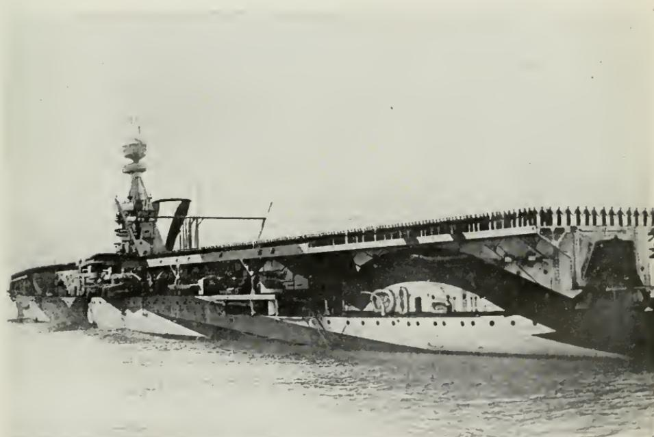
The British ship *Furious*, a "hush" cruiser, "dazzle" painted, used as a floating aérodrôme. The ship is covered with a long, broad platform upon which the aéroplanes start and alight.
