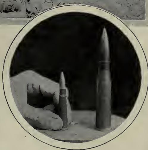
**THE ANTI-TANK BULLET COMPARED WITH AN ORDINARY BRITISH RIFLE BULLET.**
