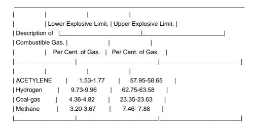
Experiments have been made at Lechbruch in Bavaria to ascertain directly the smallest proportion of acetylene which renders the air of a room explosive. Ignition was effected by the flame resulting when a pad of cotton-wool impregnated with benzoline or potassium chlorate was fired by
