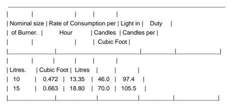
These figures indicate that the duty increases slightly with the size of the burner. Other tests showed that the duty increased more considerably with an increase of pressure, so that mantles used, or which had been previously used, at a pressure of 5 inches gave duties of 115 to 125 candles per cubic foot.
