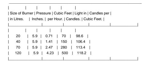
By increasing the pressure at which acetylene is introduced into burners of this type, still larger duties may be obtained from them:
